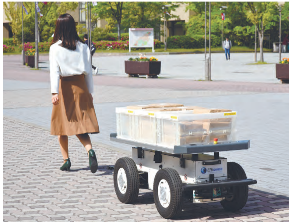
The Marble ground delivery robot follows a person at Biwako-Kusatsu Campus RITSUMEIKAN UNIVERSITY
