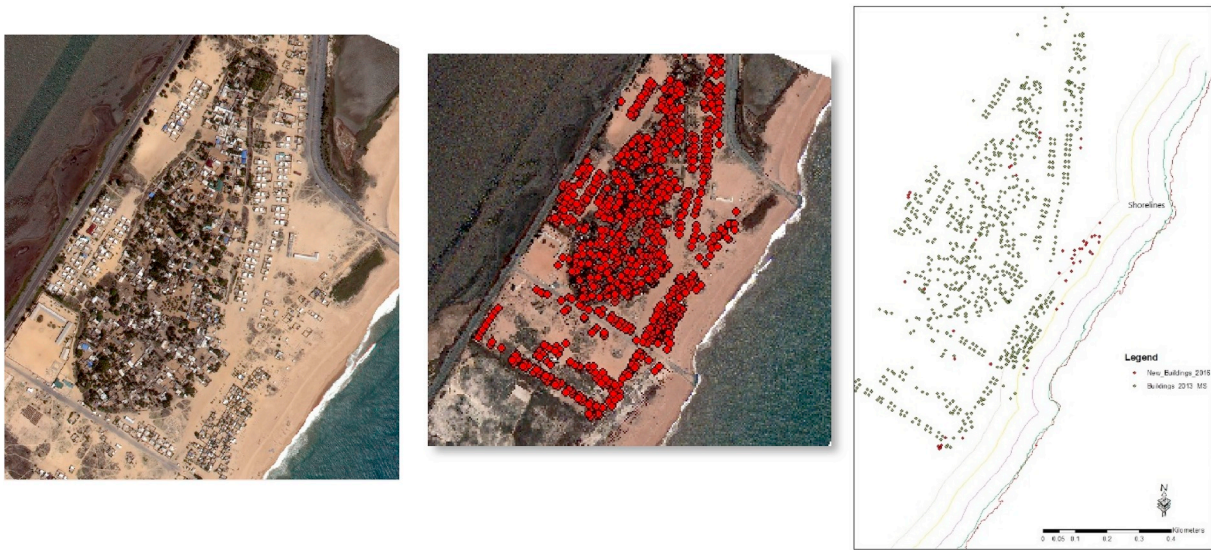
Fig. 4. Identification of housing distribution.
